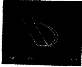
Fig. 17. Phase portrait of period 2 subharmonic motion from experimental circuit with \kappa \approx 0.09 .
