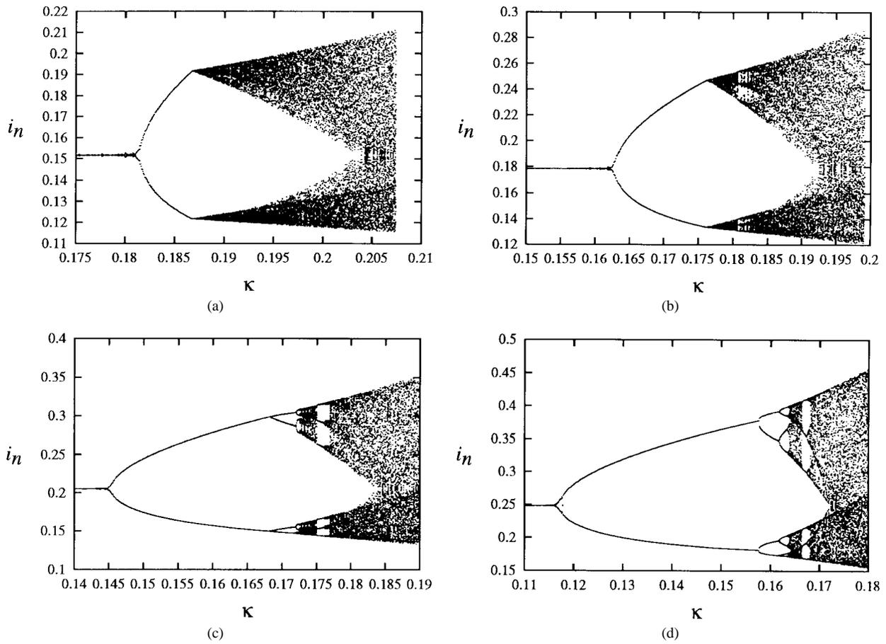
Fig. 16. Bifurcation diagrams from computer simulation of the closed-loop circuit. (a)  $I_{\text{ref}} = 0.2006\text{A}$ , (b)  $I_{\text{ref}} = 0.25\text{A}$ , (c)  $I_{\text{ref}} = 0.2918\text{A}$ , (d)  $I_{\text{ref}} = 0.3528\text{A}$ .
