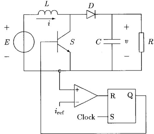
Fig. 2. Schematic of current-programmed boost converter.
