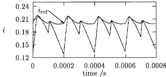
Fig. 15. Waveform of inductance current in the presence of voltage feedback loop.
