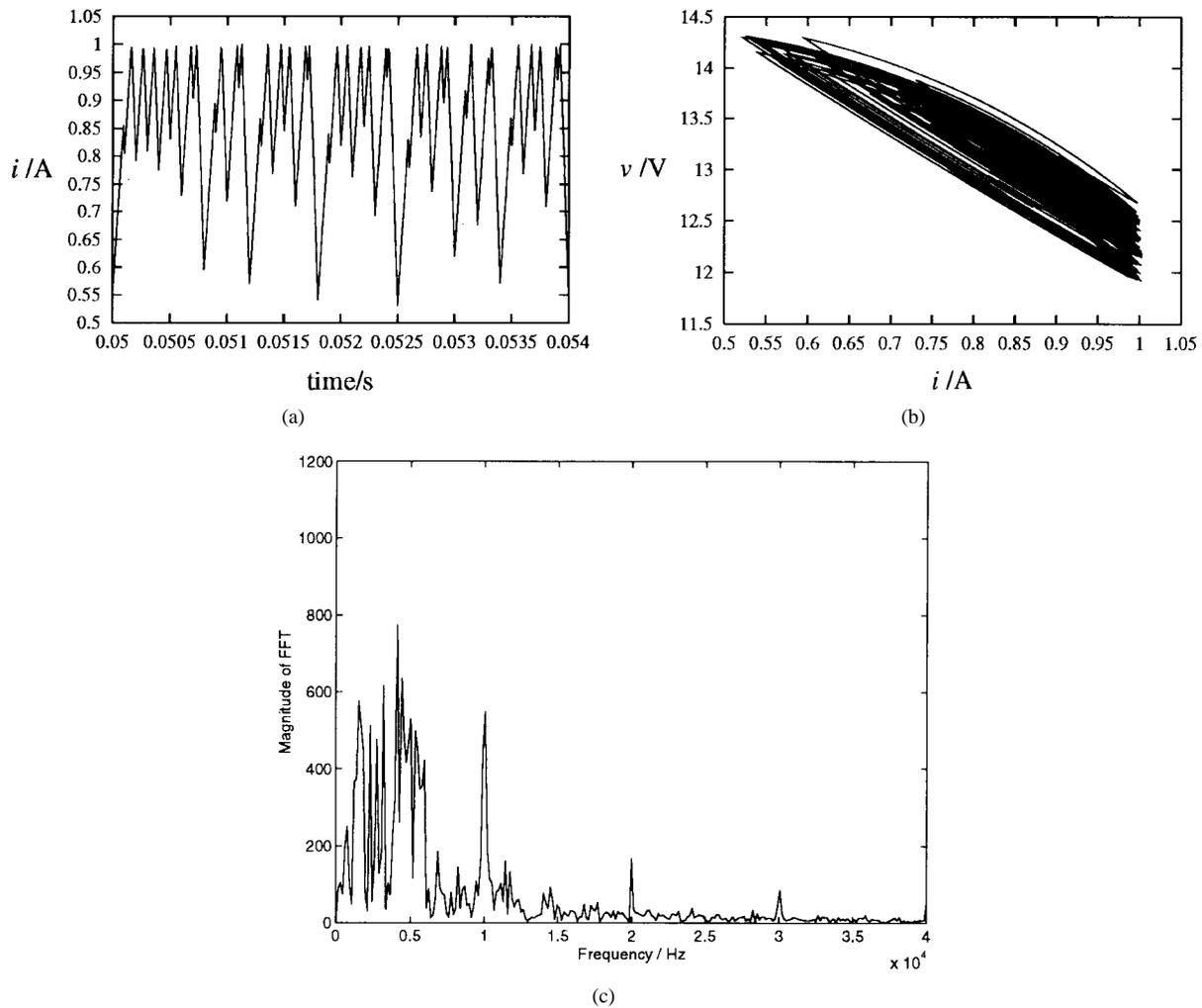
Fig. 8. Chaotic operation. (a) Time-domain waveform, (b) phase portrait, and (c) FFT spectrum of the waveform in (a).
