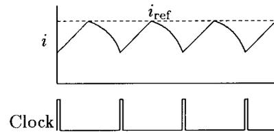
Fig. 3. Waveform of inductance current.
