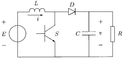
Fig. 1. The boost converter.
