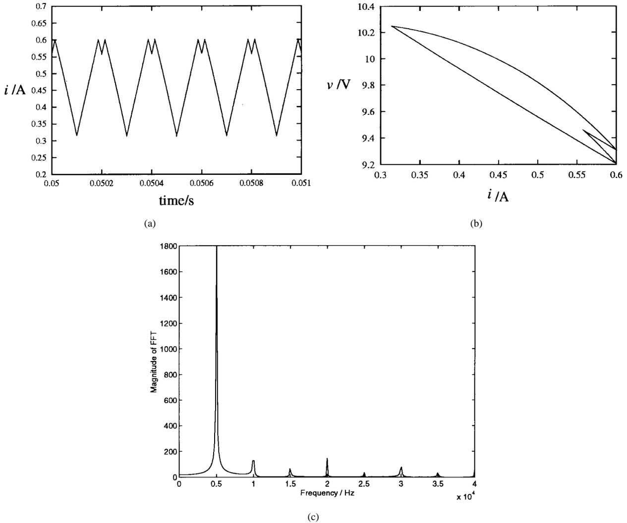
Fig. 5.  $2T$  subharmonic operation. (a) Time-domain waveform, (b) phase portrait, and (c) FFT spectrum of the waveform in (a).
