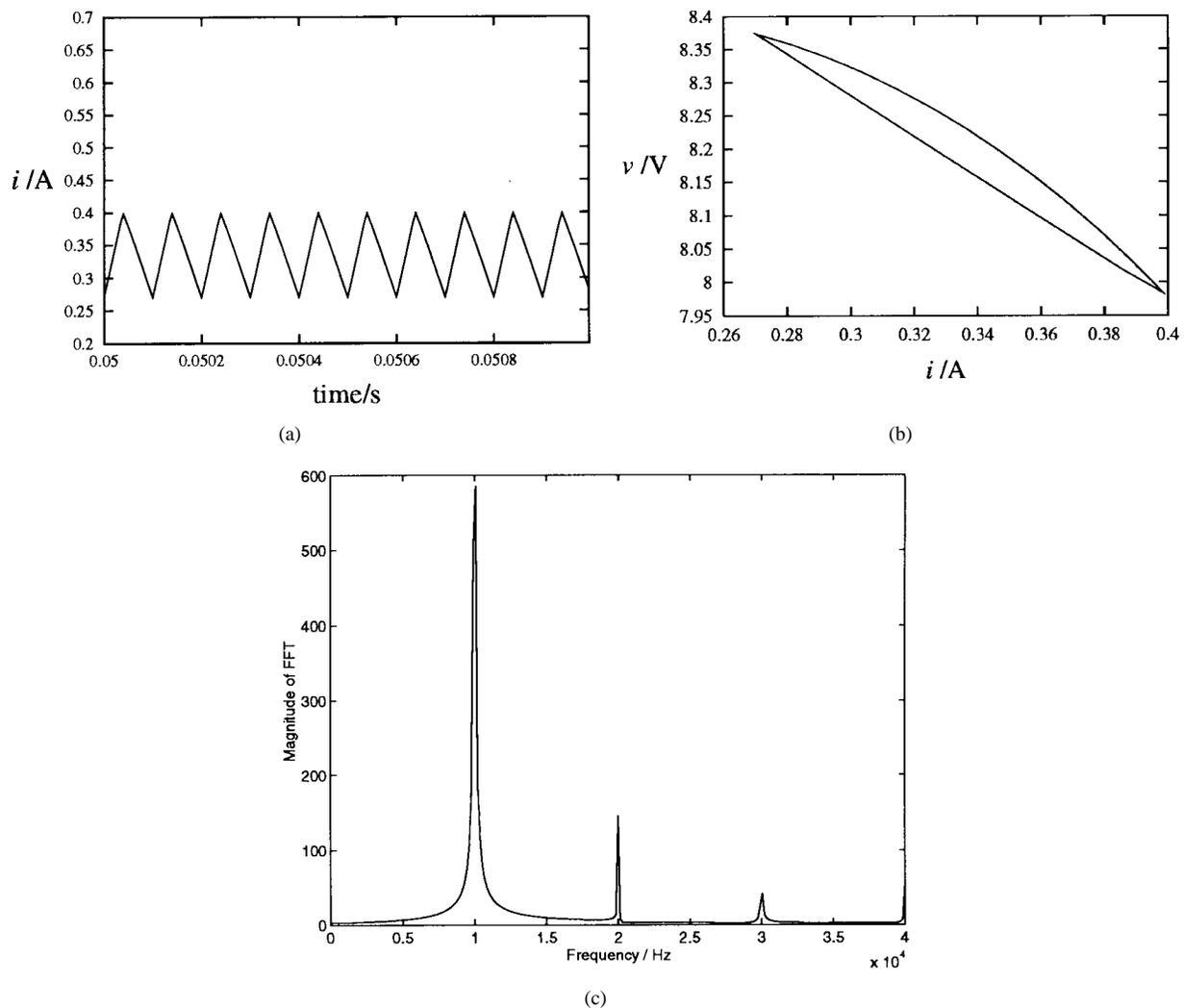
Fig. 4. Fundamental periodic operation. (a) Time-domain waveform, (b) phase portrait, and (c) FFT spectrum of the waveform in (a).
