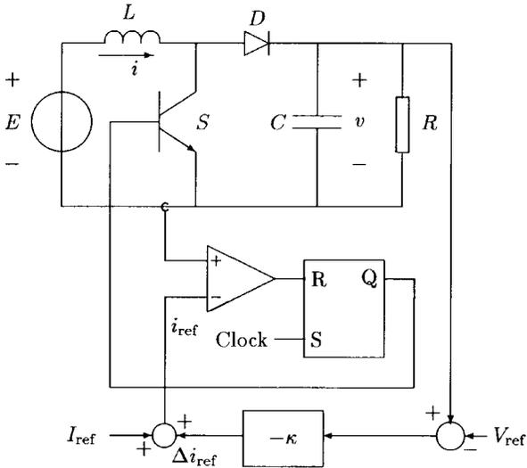
Fig. 14. Schematic diagram of the closed-loop system.
