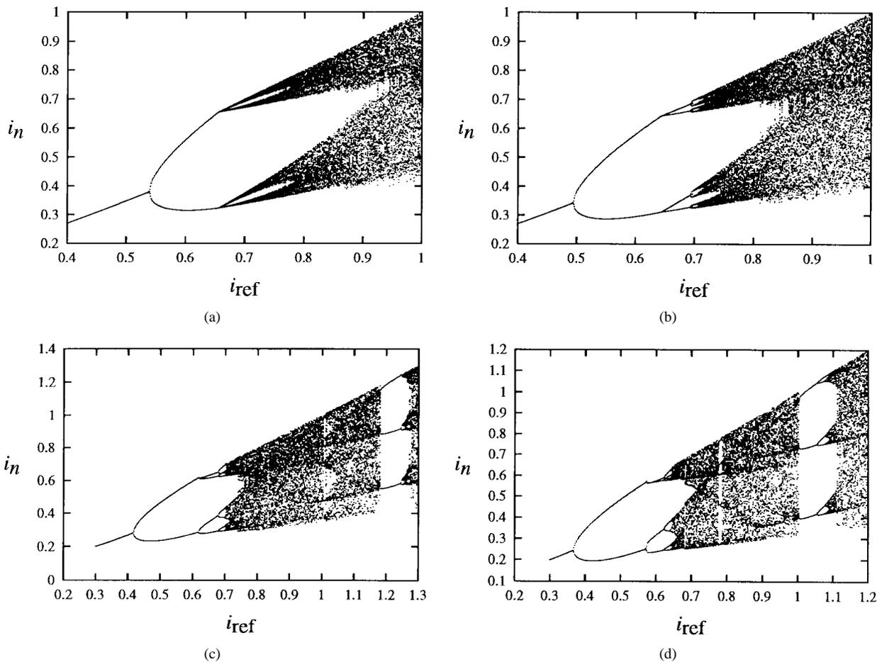
Fig. 13. Bifurcation diagrams from computer simulation of the open-loop circuit. (a)  $\gamma = 0.125$ , (b)  $\gamma = 0.25$ , (c)  $\gamma = 0.48$ , and (d)  $\gamma = 0.625$ .
