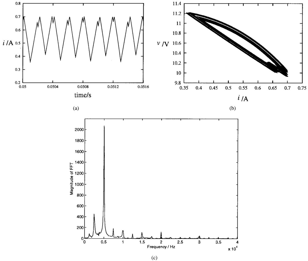
Fig. 7. Quasi- $4T$  subharmonic operation. (a) Time-domain waveform, (b) phase portrait, and (c) FFT spectrum of the waveform in (a).
