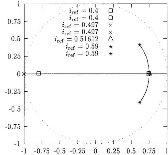
Fig. 10. Locus of characteristic multipliers for  $\gamma = 0.125$ .
