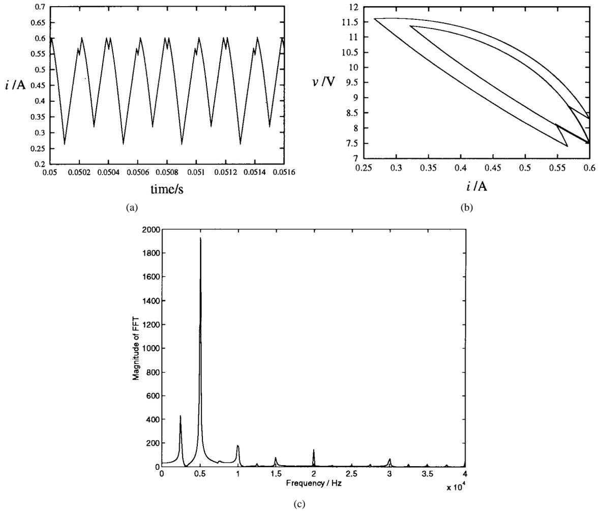
Fig. 6.  $4T$  subharmonic operation. (a) Time-domain waveform, (b) phase portrait, and (c) FFT spectrum of the waveform in (a).
