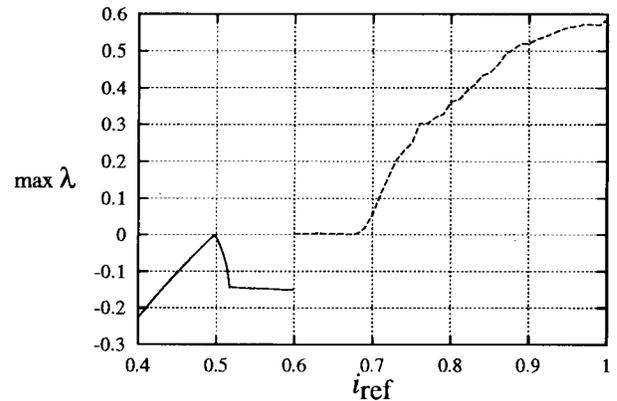
Fig. 17. The largest Lyapunov exponent versus  $i_{\text{ref}}$ , corresponding to Fig. 11(a).
