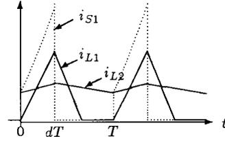
Fig. 7. Current waveforms with  $L_2$  in continuous mode.  $i_{\text{in}} = i_{L1}$  for Ćuk and SEPIC.  $i_{\text{in}} = i_{S1}$  for Zeta.
