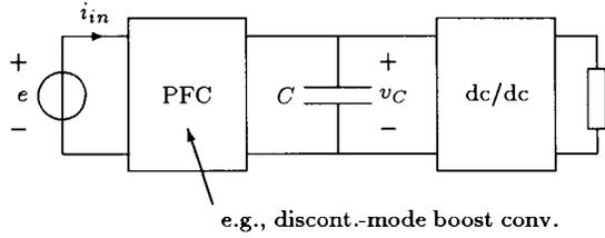
Fig. 8. Block diagram of a two-converter PFC voltage regulator.
