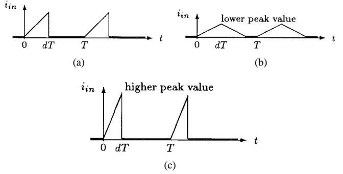
Fig. 4. Input current waveforms comparison. (a) Buck-boost converter. (b) Boost converter (lower peak). (c) Buck converter (higher peak).
