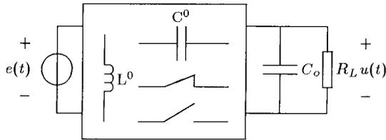
Fig. 1. Zero-order switching converter.
