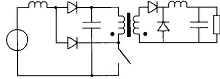
Fig. 9. Cascade of a boost converter and a buck converter to form a single-stage PFC regulator.
