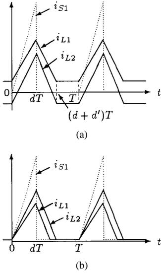
Fig. 6. Inductor currents in Ćuk, SEPIC, and Zeta converters operating in discontinuous mode (a) without and (b) with additional diodes in series with inductors.
