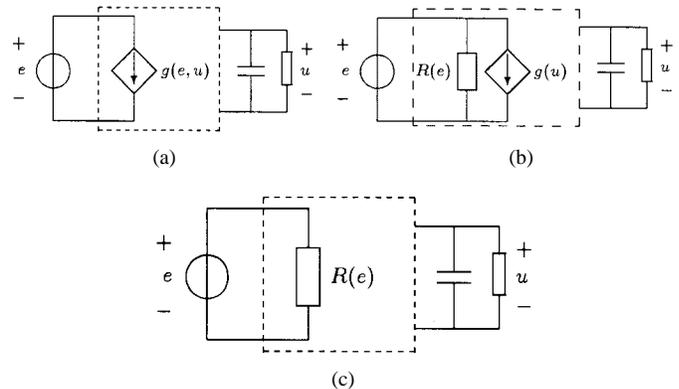
Fig. 3. Averaged models of impedance. (a) General model. (b) Variable separable. (c) zero-order impedance (resistive). Dependence on  $d$  and  $T$  of all functions omitted for brevity.
