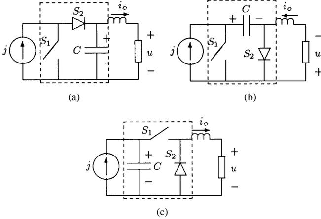
Fig. 10. Zero-order and near zero-order switching converters based on  $C^0$ . Direct duals of (a) buck. (b) Buck-boost. (c) Boost converters.
