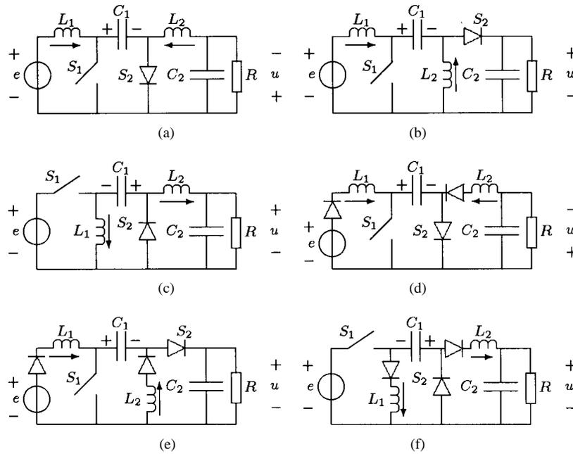
Fig. 5. Higher order converters. (a) Ćuk converter. (b) SEPIC converter. (c) Zeta converter. (d)–(f) Converters with additional diodes to create  $L^0$ .
