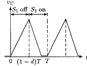
Fig. 11. Capacitor voltage waveform for circuits of Fig. 10.
