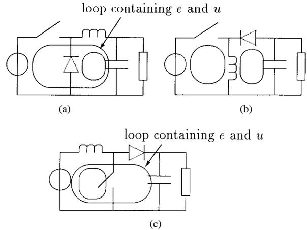
Fig. 2. Corollary 1. (a) Buck converter has a loop that contains input port and output port. (b) Buck-boost converter has no such loops. (c) Boost converter has such a loop.
