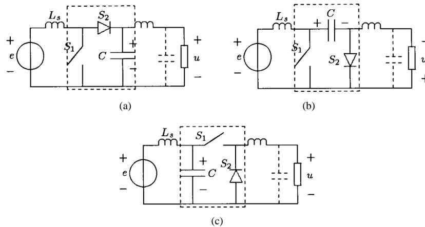
Fig. 12. Modified dual converters for practical source and load. Capacitor  $C$  operates in discontinuous mode.
