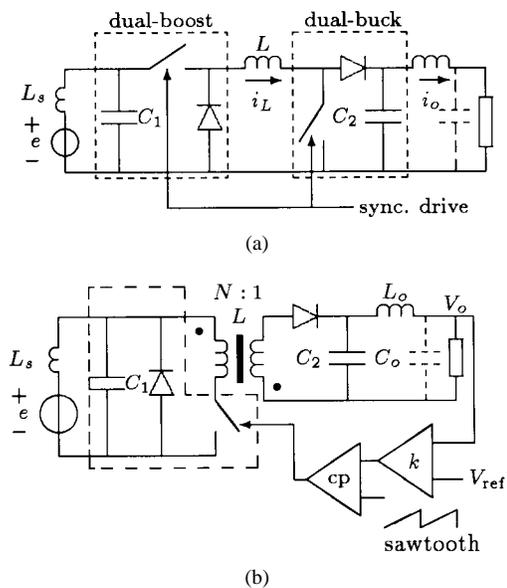
Fig. 13. (a) Dual single-stage PFC regulator with  $C_1$  in discontinuous mode; switches are synchronized for single-stage operation. (b) Isolated version.
