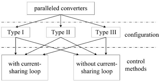
Fig. 4. Systematic classification of parallel connected converters.
