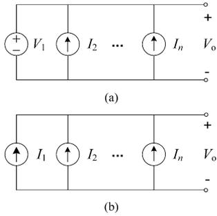
Fig. 1. Structures for paralleling ideal independent sources.
