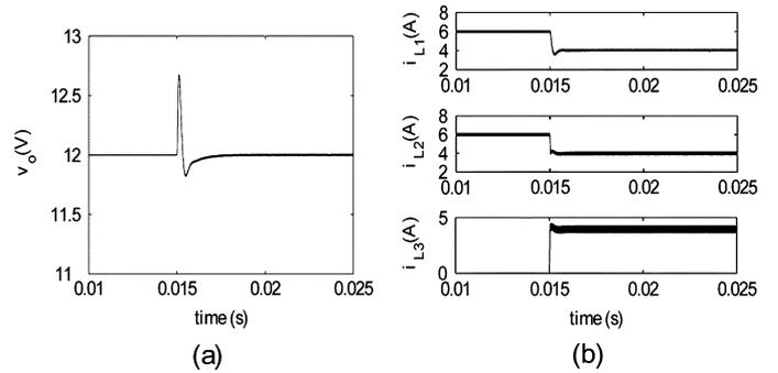
Fig. 15. Simulation results for plug-in transient for Type-II scheme without current-sharing loop. (a) Output voltage. (b) Converter output currents.
