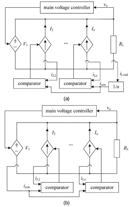
Fig. 7. Control structures for Type-II configuration (a) without current-sharing loop, and (b) with current-sharing loop (also known as master-slave current sharing).
