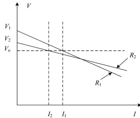
Fig. 5. Output characteristics of two parallel connected converters.
