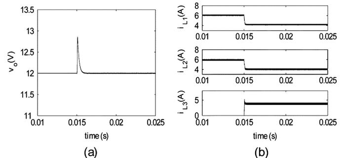
Fig. 21. Simulation results for plug-in transient for Type-III scheme with current-sharing loop. (a) Output voltage. (b) Converter output currents.
