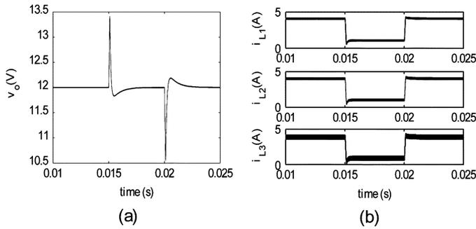
Fig. 16. Simulation results for stepped load for Type-II scheme with current-sharing loop. (a) Output voltage. (b) Converter output currents.
