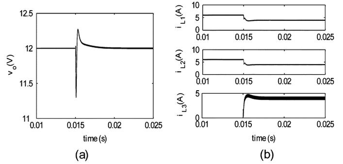
Fig. 13. Simulation results for plug-in transient for Type-I scheme with current-sharing loop. (a) Output voltage. (b) Converter output currents.
