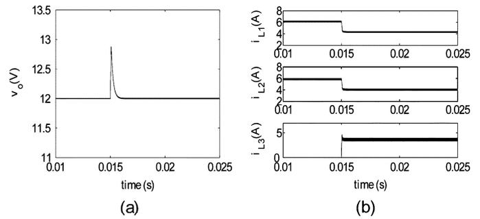
Fig. 19. Simulation results for plug-in transient for Type-III without current-sharing loop. (a) Output voltage. (b) Converter output currents.
